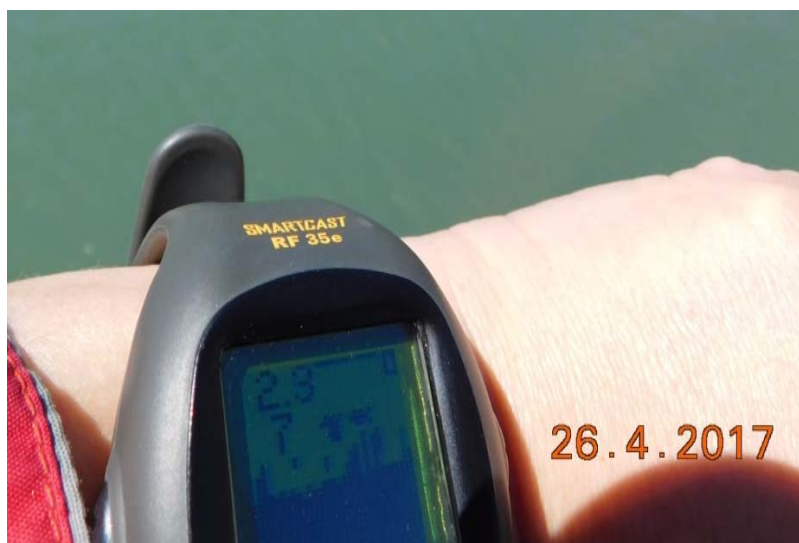
Figure 5. Study of the fish distribution using echo depth-sounder
