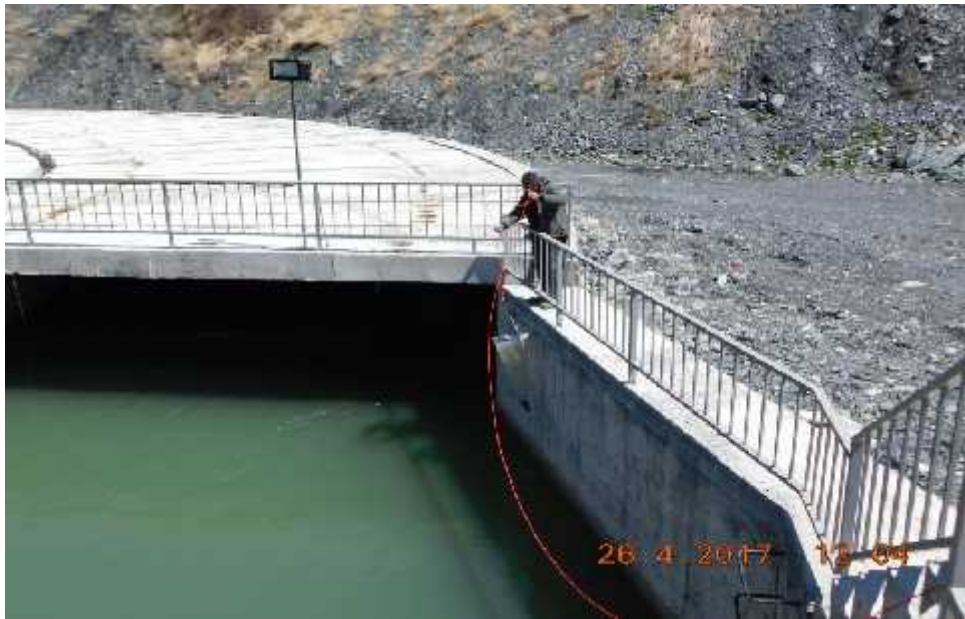
Figure 3. Insert of the cone net into water reservoir
